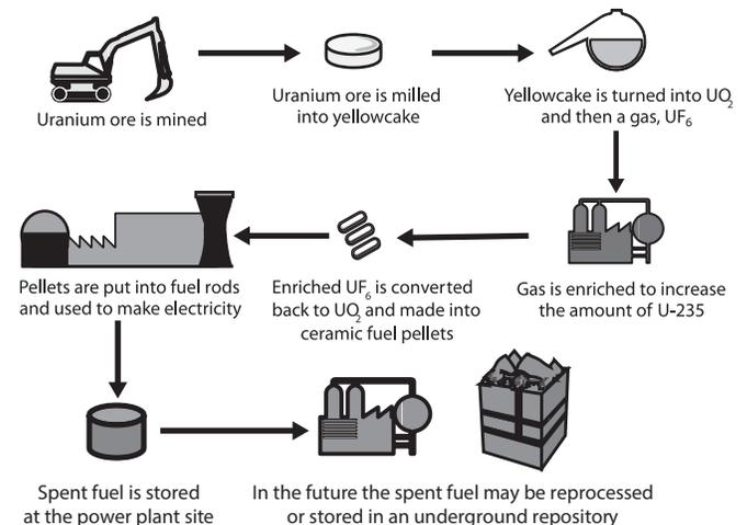
spent fuel is usually stored near the reactor in a deep pool of water called the spent fuel pool. The spent fuel cools and loses most of its radioactivity through radioactive decay. In three months, the spent fuel will lose 50 percent of its radiation; in one year, 80 percent; in 10 years, 90 percent. The spent fuel pool was intended as a temporary method for storing used nuclear fuel. However, there is no permanent storage solution yet for spent fuel, and space in fuel pools is running out.
